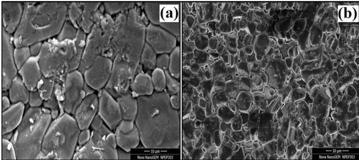
Figure 4: (a) FESEM image of pure ZnO thin film (b) FESEM image of MgO incorporated ZnO thin film
