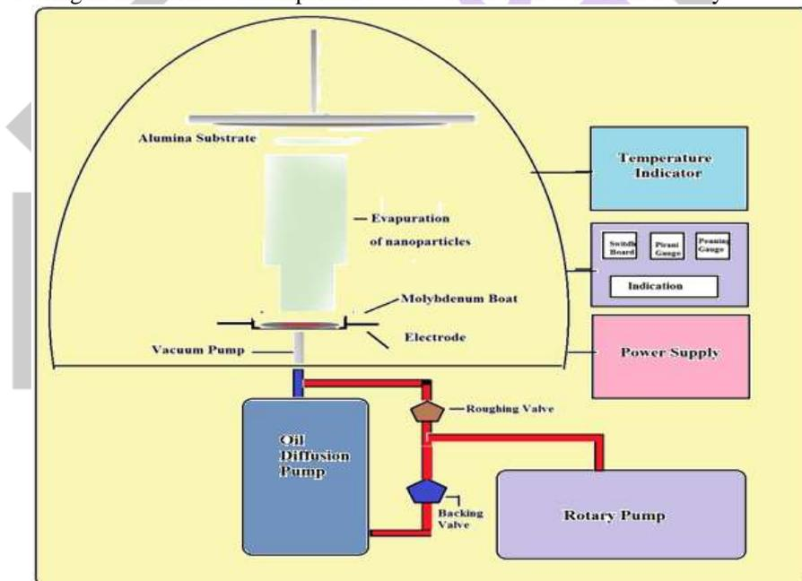
Figure 2: Thermal Evaporation system
