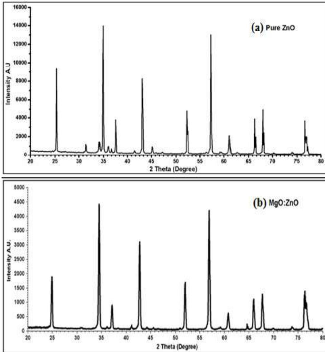
Figure 3: (a) XRD pattern of pure ZnO thin film (b) XRD pattern of MgO incorporated ZnO thin film
