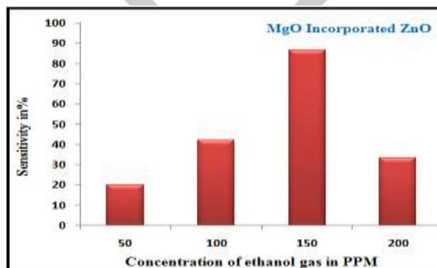
Figure 7: Sensitivity verses ethanol gas concentration in PPM.
