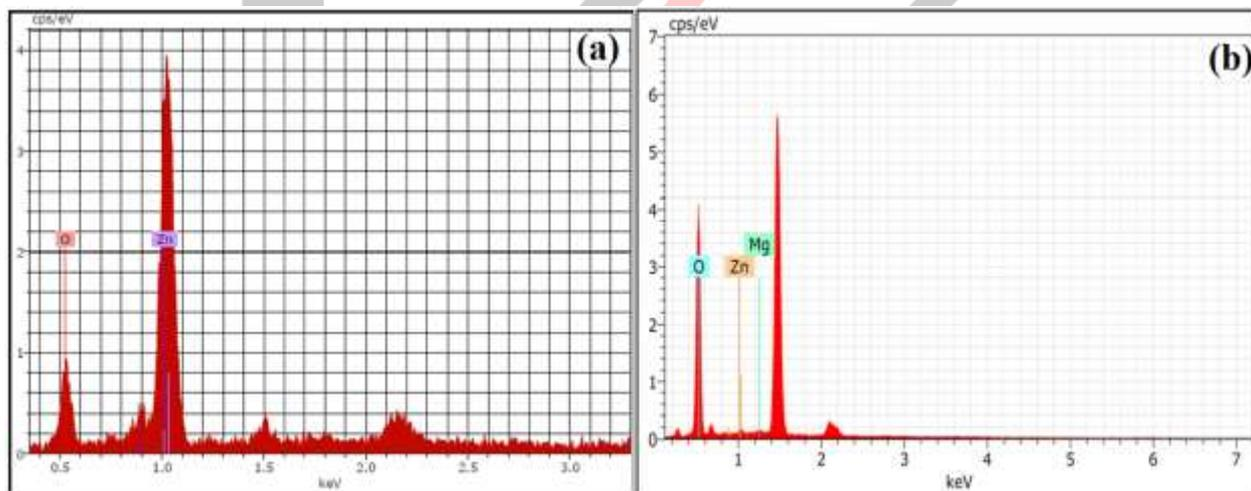
Figure 5: (a) EDS of pure ZnO thin film (b) EDS of MgO incorporated ZnO thin film
