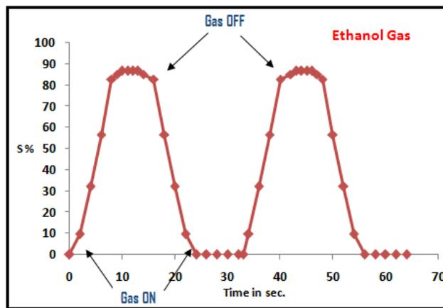
Fig. 8 Response and recovery time of MgO incorporated ZnO nanostructured binary oxide thin films
