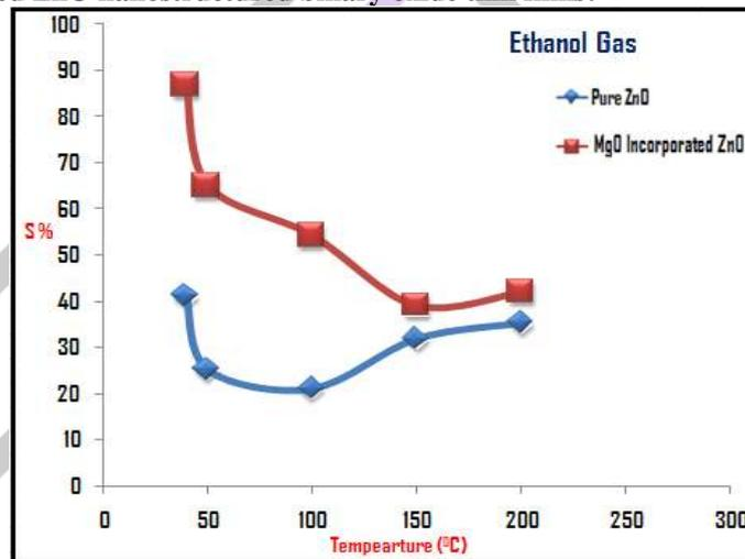
Figure 6: Sensitivity of MgO incorporated ZnO nanostructured binary oxide thin films
